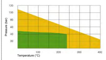
The P x T diagram above indicates the service limits for **NA** -1005 considering the simultaneous influence of pressure and temperature (chemical suitability assumed). The green area represents the normal service limits, while the orange coloured area shows the maximum application limits. For those cases, please consult our technical department.
