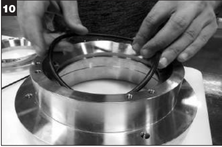
10 Remove O-Ring from gland inside diameter and discard.
