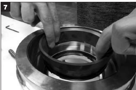
7 Invert gland assembly and remove stationary seal ring and discard.
