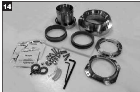
14 Remove spare parts kit components from packaging and place on a clean work surface. NOTE: Leave the two largest O-Rings packaged for size identification.
