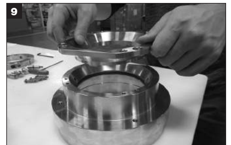
9 Invert gland assembly. Remove shoulder screws and discard. Lift pusher from gland assembly.
