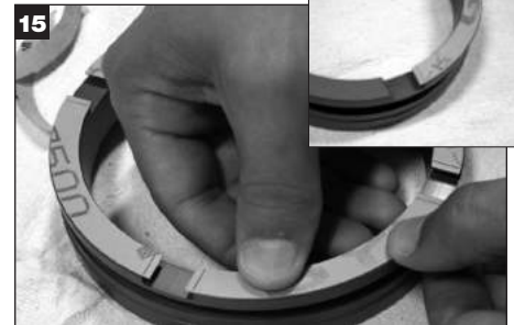
15 Place the rotary seal face on a dry clean cloth face side down to avoid scratching or damaging the face. Peel the adhesive backing from the rotary cushions. Align scored edges with edges of slots and press to ensure adhesion to that surface.
