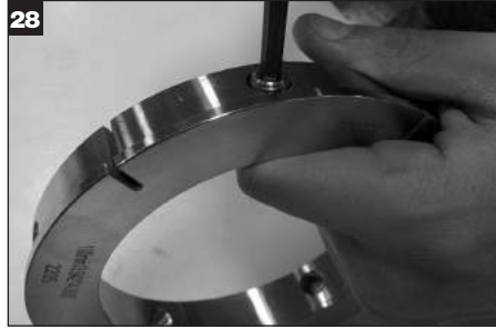
Install dog point and TORX screws into lock ring.
