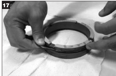
17 Apply a thin film of grease to the rotary O-Ring and install in the rotary seal face outside diameter groove
