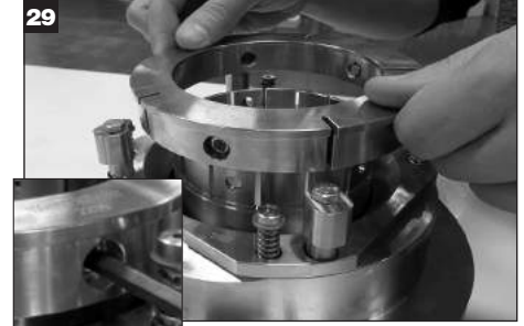
Slide the lock ring over the sleeve. Align dog point screw holes in the lock ring with holes in the sleeve. Tighten dog point screws until flush with inside diameter of sleeve.
