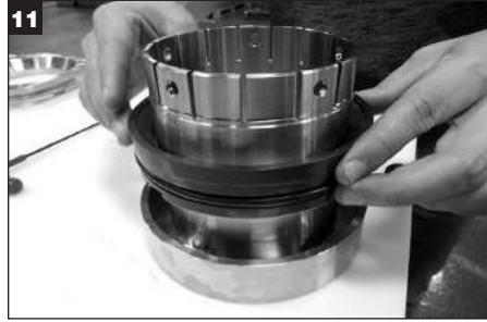
11 Remove rotary seal ring from sleeve and discard.
