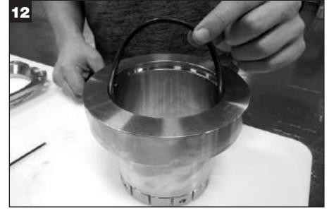
12 Remove shaft O-Ring from sleeve inside diameter and discard.
