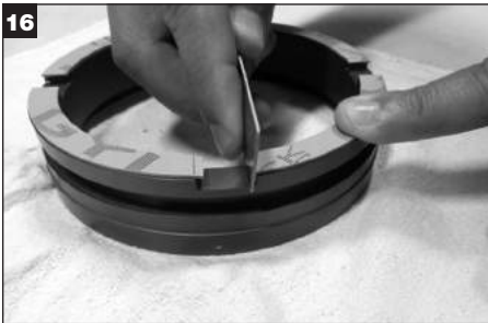
16 Fold the cushion tabs into the slots and press them in against the drive slot edge with a straight edged tool or ruler.
