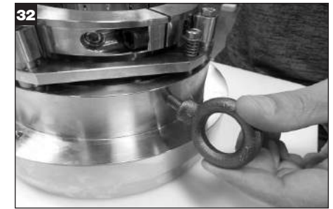
Install eye bolts for ease of transportation. IMPORTANT: Remove eye bolts prior to seal installation.
