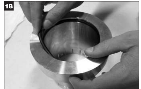
18 Apply a thin film of grease to the shaft O-Ring and install in the sleeve inside diameter groove.
