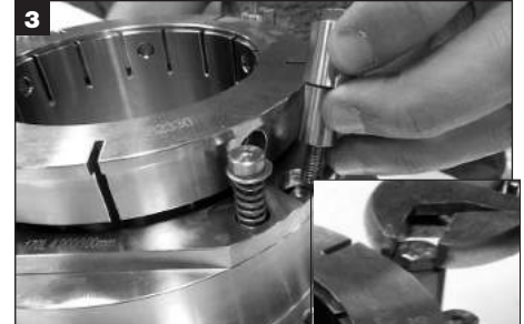
3 Disengage centering clips and remove screws, clips, and bushings from pusher and discard.
