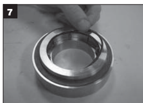
EN Install O-Ring in gland
