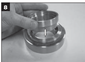
EN Insert stationary holder into gland
