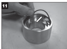
EN Install rotary holder O-Ring
