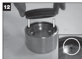
EN Install rotary face in holder (Line up slots with lugs)
