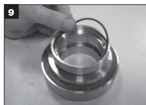
EN Install stationary holder O-Ring
